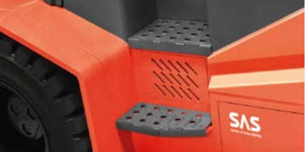
The low and wide steps and large driver assist grip ensure operator fatigue is minimized in applications that require repeatedly getting in and out of the truck
