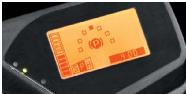
The steering wheel direction indicator shows the rear wheels' alignment to the operator at a glance
