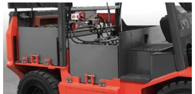
Easy 'lift out' battery extraction
